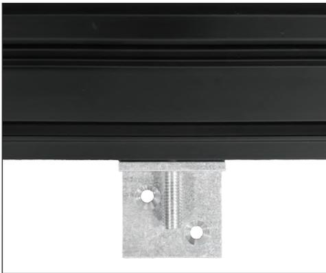
Prepare the install location to ensure your frame will be accurately placed. Begin by marking the intended install location for the top wall mount brackets. Each cut length will receive 2 wall mount brackets, depending on size. Ensure the top of each bracket is level and the screw is through the top at least 1/4 inch. Secure the bracket to the wall and test the frame by hanging it on top of the brackets. If necessary adjust the screw to level the frame.
