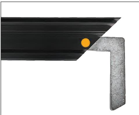
**Insert** one pair of corner brackets into the open channel on two adjoining corner ends of the aluminum extrusion, sliding in to create a corner or 90 angle. Slightly tighten the screws and repeat for the remaining corners..
