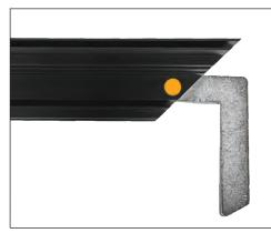
Insert one pair of corner brackets into the open channel on two adjoining corner ends of the aluminum extrusion, sliding in to create a corner or 90 angle. Slightly tighten the screws and repeat for the remaining corners..
