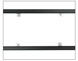
Once your frame is level and the top mounting brackets have been installed, add the bottom wall mount brackets to finish securing the frame. Each length will have 2 wall mount brackets, depening on size. The sides of your frame may not have wall mount brackets but additional can be installed for additional security, usually only on very large frames. Once complete your frame should be secure and snug to the wall.
