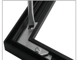
Insert one pair of corner brackets into the open channel on two adjoining corner ends of the aluminum extrusion, sliding in to create a corner or 90 angle. Slightly tighten the screws and repeat for the remaining corners. Tighten completely when the frame is finished
