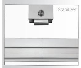
Match your stabilizer lengths with coordinatig expansion hardware. Slide the expansion hardware into the stabilizer end and slightly tighten the set screw to hold into place. Now slide that end into the inside frame channel, once in place next to the seam, tighten the screw until secure.
