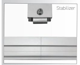
Match your stabilizer lengths with coordinatig expansion hardware. Slide the expansion hardware into the stabilizer end and slightly tighten the set screw to hold into place. Now slide that end into the inside frame channel, once in place next to the seam, tighten the screw until secure.
