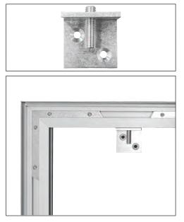
**Prepare** the install location to ensure your frame will be accurately placed. Begin by marking the intended install location for the top wall mount brackets. Each cut length will receive 2 wall mount brackets, depending on size. Ensure the top of each bracket is level and the screw is through the top at least 1/4 inch. Secure the bracket to the wall and test the frame by hanging it on top of the brackets. If necessary adjust the screw to level the frame.
