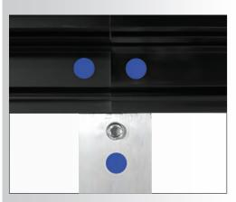
Match your stabilizer lengths with coordinatig expansion hardware. Slide the expansion harware into the stabilizer end and slightly tighten the set screw to hold into place. Now slide that end into the inside frame channel, once in place next to the seam, tighten the screw until secure.
